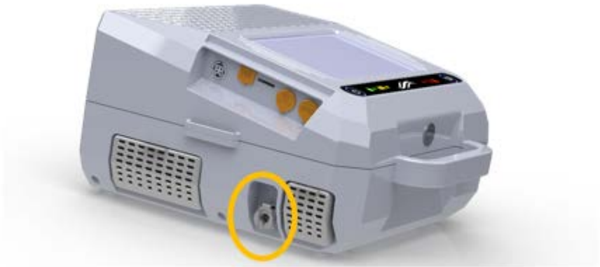
Figure 14 Connecting an External Oxygen Source
