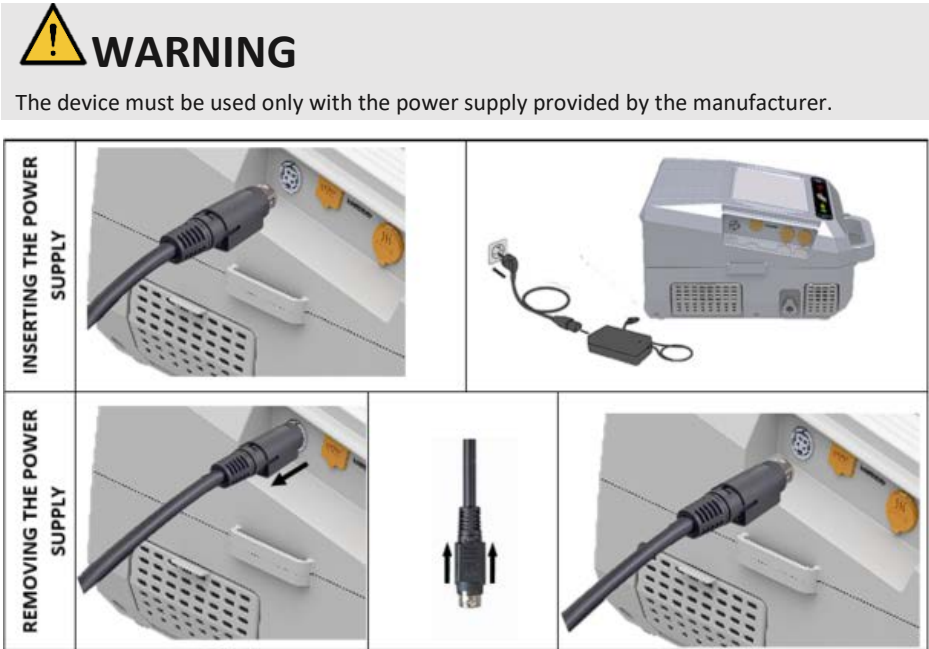
Figure 10 Power Supply Inserting and Removing
