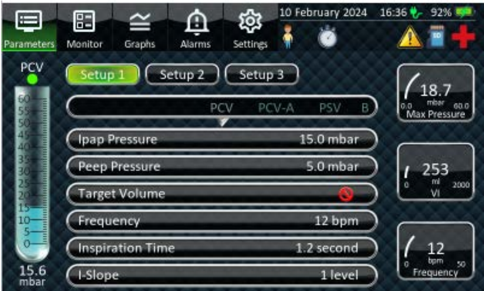
Figure 21 Ventilation Operating Mode Selection and Parameter Settings
